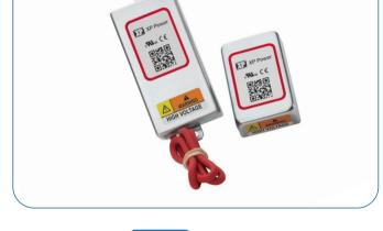
The C Series is a line of miniature, regulated high voltage power supplies. Each model is programmed from 0 to 100% of rated output via a 0 to +5 volt, DAC-compatible, high-impedance programming input voltage. An externally accessible potentiometer provides adjustable gain trim, allowing for individual calibration of units.
