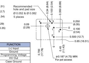
All grounds internally connected except case. Case ground (Pin5) must be connected to ground, with no more than 50V between case ground (Pin 5) and circuit ground (Pin 2).
